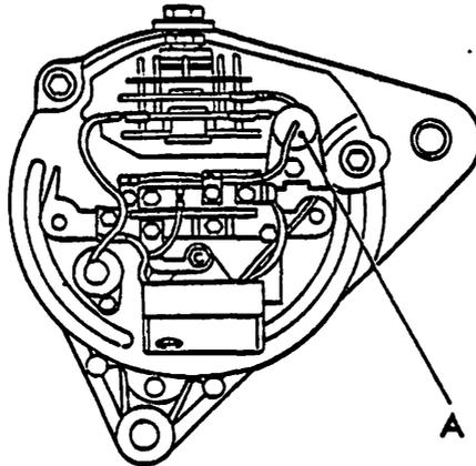
If the alternator output falls to zero, the fault may be caused by a short circuit of the surge protection diode (A); to check this, proceed as follows:-(NOTE 18 ACR ILLUSTRATED)
