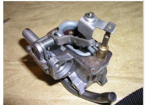
Now slide the operating lever on its pivot to the left (outside) to clear the metering bracket.
