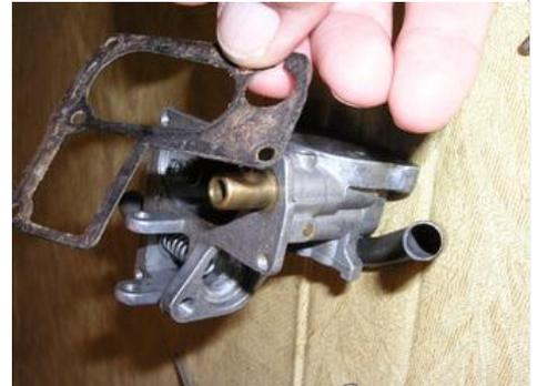
With the operating lever removed, you can remove the gasket safely. Remove the thermostatic actuator return spring, bushing and sleeve.
