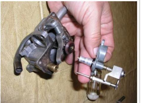
...and remove it from the body. This is as far as you should need to go with disassembling the air valve casting. The
