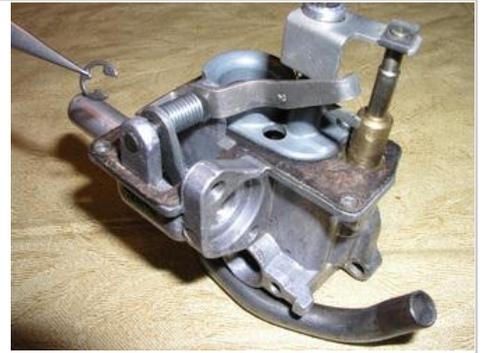
The E-clip removed. The outlet tube is just propping up the unit so it won't fall over while I photograph it.
