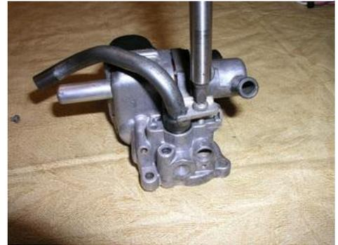
Now remove the pozidrive screw holding the clamp to the outlet tube...
