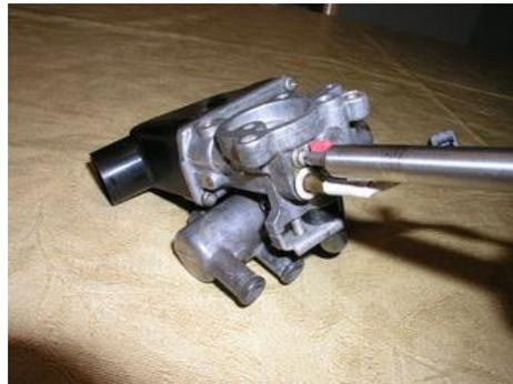
Begin the disassembly by removing the cartridge heater. This gets the wires, which are often brittle, out the way and prevents further damage. Remove the pozidrive screw and the heater should pull out...
