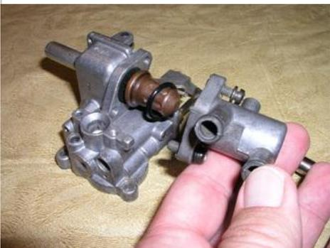
Withdraw the water cell and reveal the thermostat bulb and O ring. Be sure the bleed screw on the water cell is clear. You will need to bleed air from the water cell with the engine running once everything is back together. The thermostatic actuator will not work if there's air in the water cell, and it will not bleed itself. If you find the unit needs to be bled constantly to keep it functioning, you don't have an FASD problem, you have a head gasket problem.
