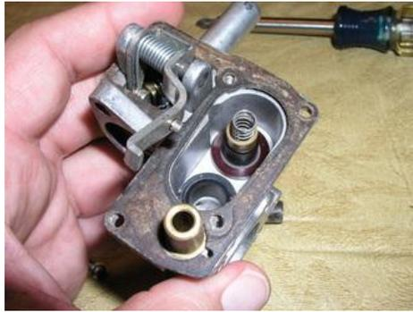
This spring can be left in place unless it falls out. It's often stuck in there good and you don't want to stretch it while removing it. Better to simply clean it by soaking it where it is. That plastic bushing comes out easily.
