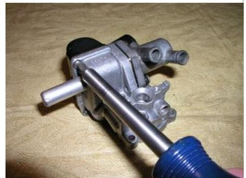
Remove the three pozidrive screws holding the snorkel cover on and remove it.
