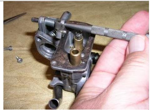
Once the ridged bit at the end of the pivot is clear of the casting, you should be able to remove it by hand.
