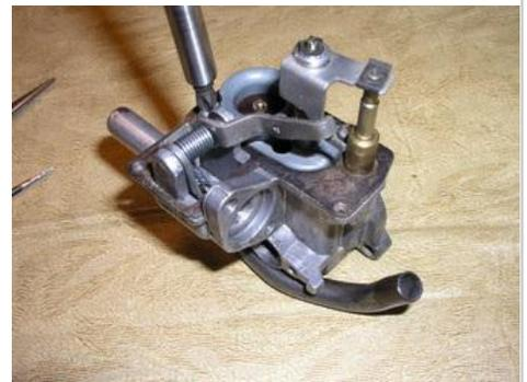
Remove the two pozidrive screws securing the air valve casting to the FASD body...
