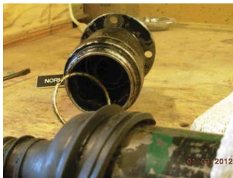
Locking ring removed from the CV joint, new boot installed
